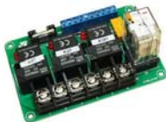
PCB ; POWER/STEP RELAY
